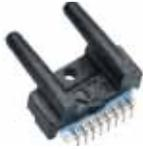
**Airflow sensors:** Advanced microstructure technology. Sensitive and fast response to flow, amount/direction of air or other gas. Proportional output voltage. Thin-film, thermally isolated bridge structure consists of a heater and temperature sensing elements. **May be used in:** HVAC, respirators, process control, oxygen concentrators, gas metering, chromatography, leak detection equipment, medical/analytical instrumentation, and ventilation equipment.
